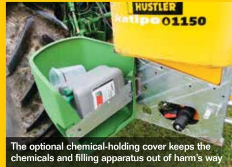
The optional chemical-holding cover keeps the chemicals and filling apparatus out of harm's way
