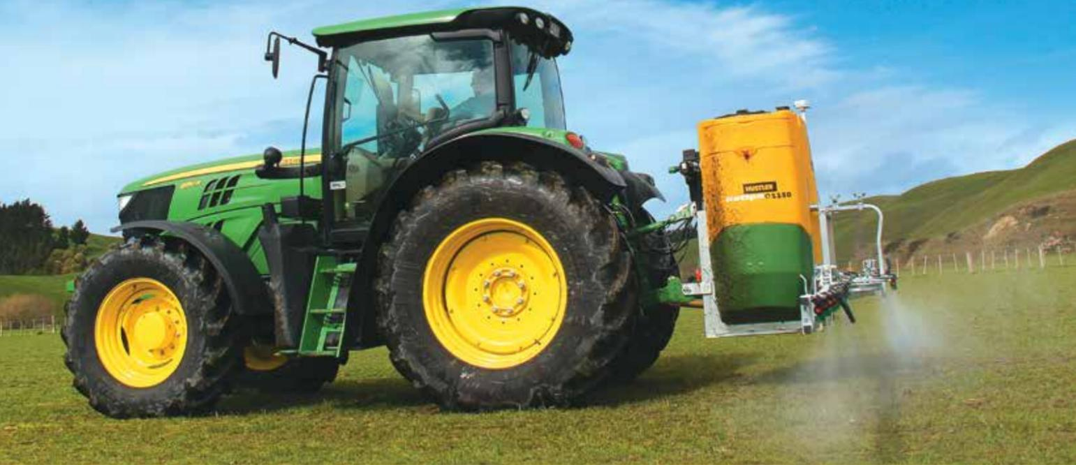
The hand-wash tank has a capacity of 18L and a little tap at the bottom to make washing your hands easy, while an optional 100L clean-water rinse tank can completely rinse the tank in under a minute. This is located under the green cover on the right-hand side of the tank, which is handy for those using a lot of different sprays to ensure Farmer Brown's nice lush grass gets the liquid fertiliser and not the roundup treatment you were spraying at the previous job.
