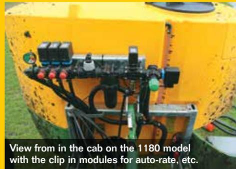
View from in the cab on the 1180 model with the clip in modules for auto-rate, etc.
