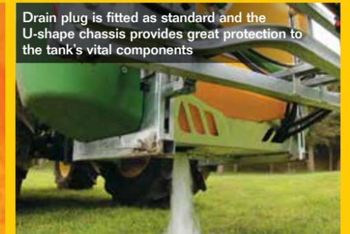
Drain plug is fitted as standard and the U-shape chassis provides great protection to the tank's vital components
